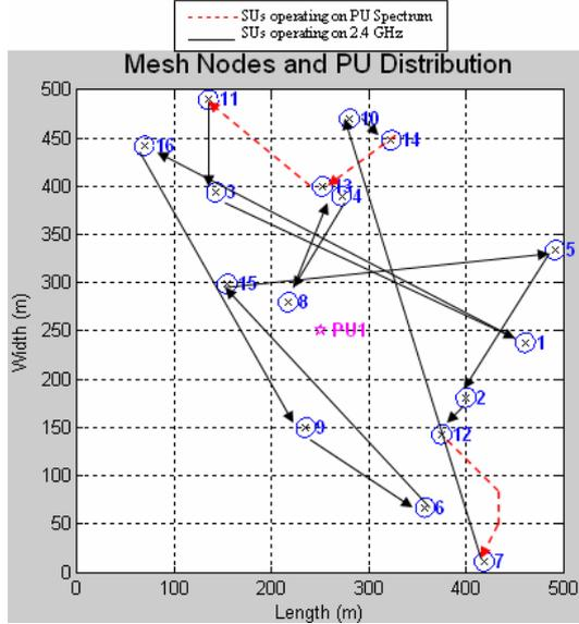
Figure 3. Communication between SU nodes on the IEEE 802.11 and licensed spectrums (scenario 2).
